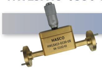
The HASCO **HWLSA15-0330-ER** is an V Band Level Set Waveguide Attenuator and covers a frequency range of **50 to 75 GHz**. This attenuator is equipped with a micrometer dial which makes the dB value mechanically adjustable. This attenuator is ideal for a waveguide system where broadband level setting is required. It is a passive, reciprocal network where either side can serve as input.
